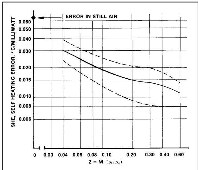
Figure 13: Wind Tunnel Data; Model 102 Self-heating Errors
