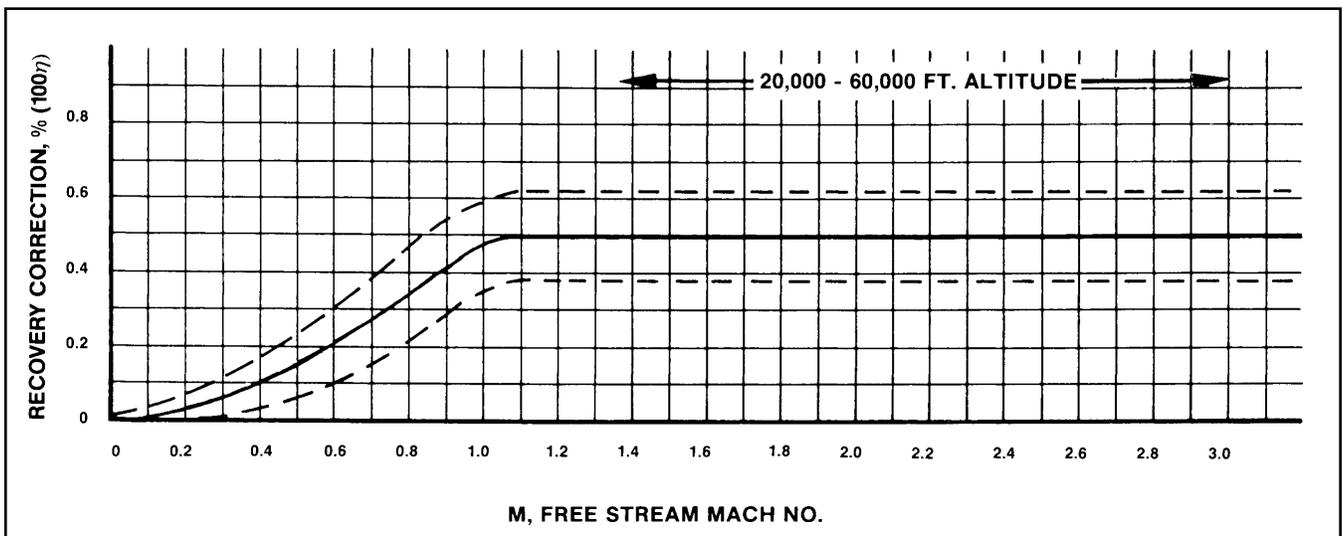
Figure 7: Wind Tunnel Data; Model 101 Recovery Corrections
