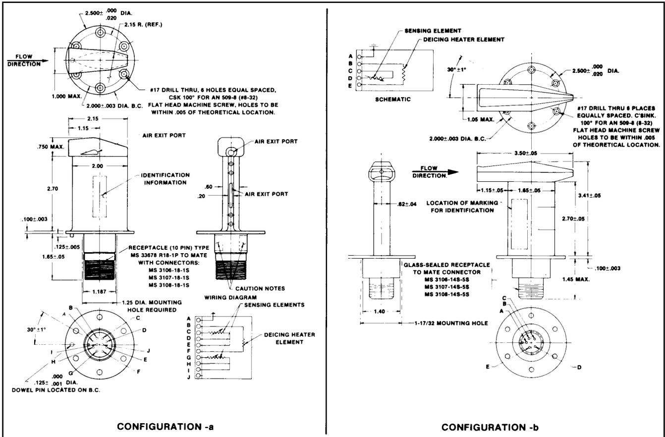
Figures 11-A, -B: Deiced Model 102 Standard Configurations
