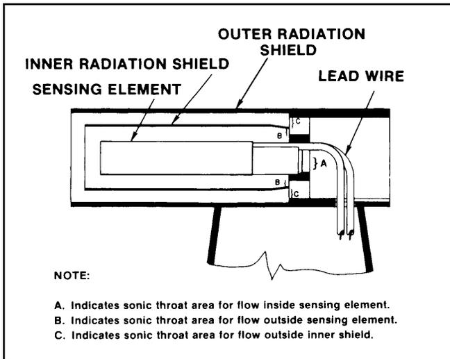
Figure 4: Cross Section of Model 101 Sensor Head
