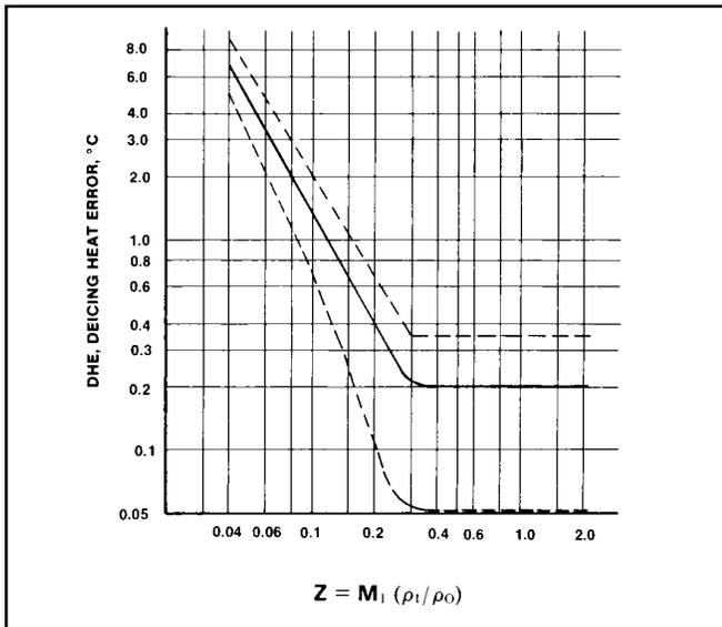
Figure 15-A: Wind Tunnel Data; Deicing Heat Errors for Model 102 Sensors, Single Mandrel Construction (1 or 2 Elements)
