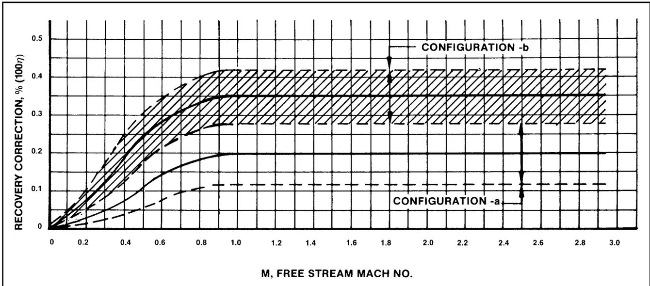
Figure 14: Wind Tunnel Data; Model 102 Recovery Corrections
