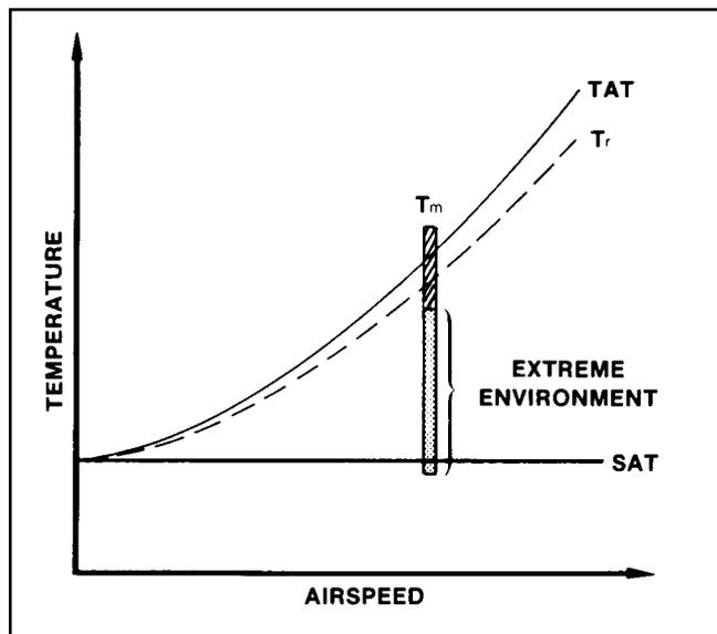
Figure 1: Temperature Relationships in Flight
