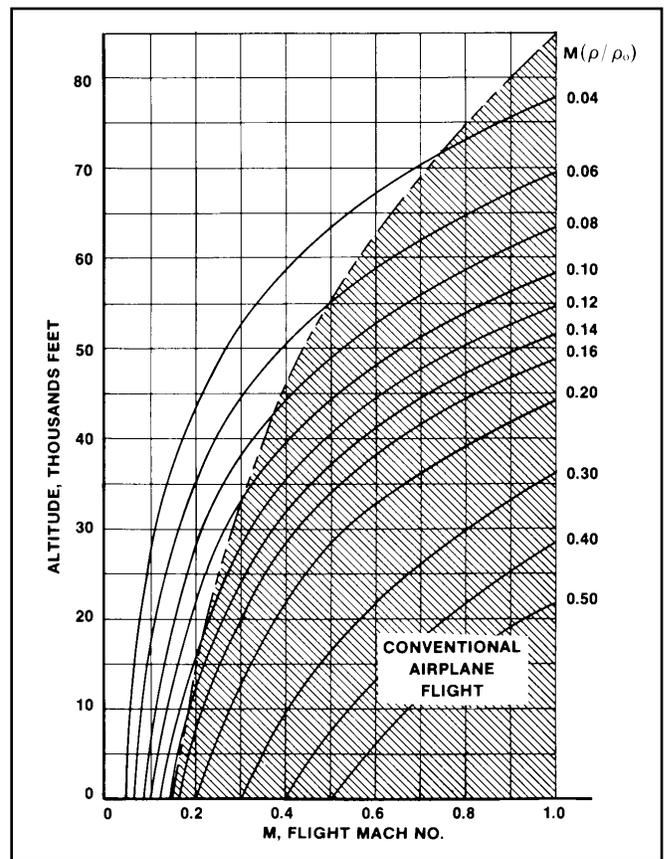
Figure 2: Subsonic Flight in U.S. Standard Atmosphere
