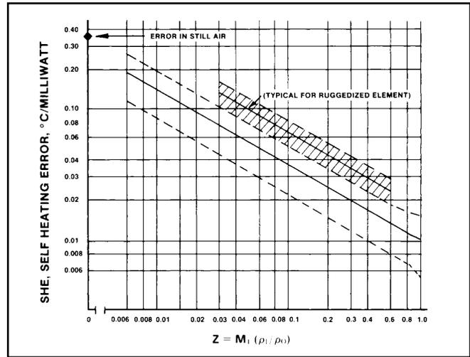
Figure 21: Wind Tunnel Data; Non-deiced Model 102 (Open-wire Element) Self-heating Errors
