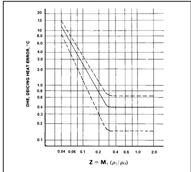
Figure 15-B: Wind Tunnel Data; Deicing Heat Errors for Model 102 Sensors, Dual Mandrel Construction (Multiple Elements)
