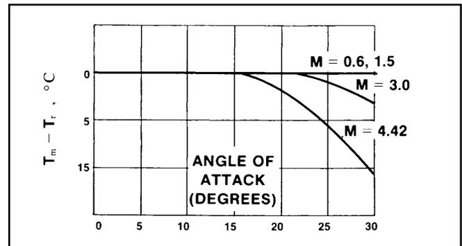
Figure 8: Airflow Direction Sensitivity
