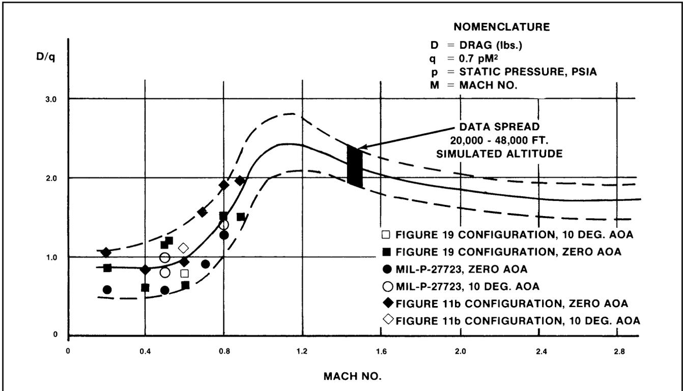
Figure 24: Wind Tunnel Data; Drag of Deiced and Non-deiced Model 102 Sensors
