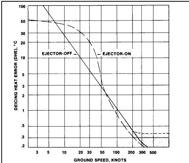
Figure 18-A: DHE Versus Constant Values of Ground Speed
