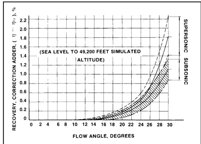
Figure 22: Wind Tunnel Data; Non-deiced Model 102 Flow Angle Sensitivity in Subsonic and Supersonic Flow
