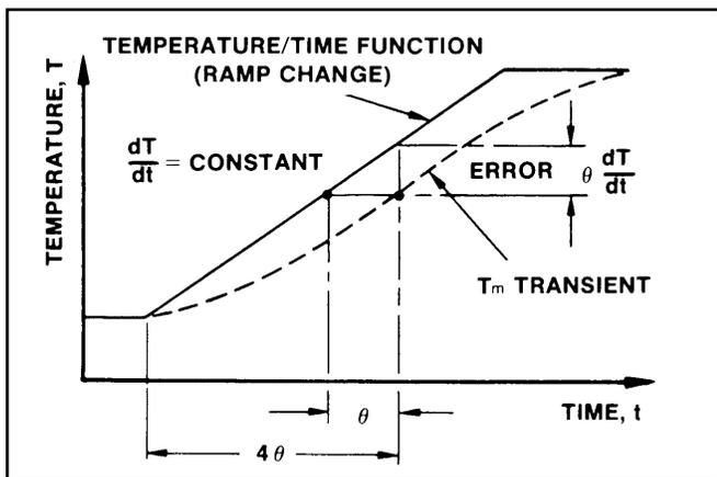
Figure 3-B: Temperature/Time Function (Ramp Change)
