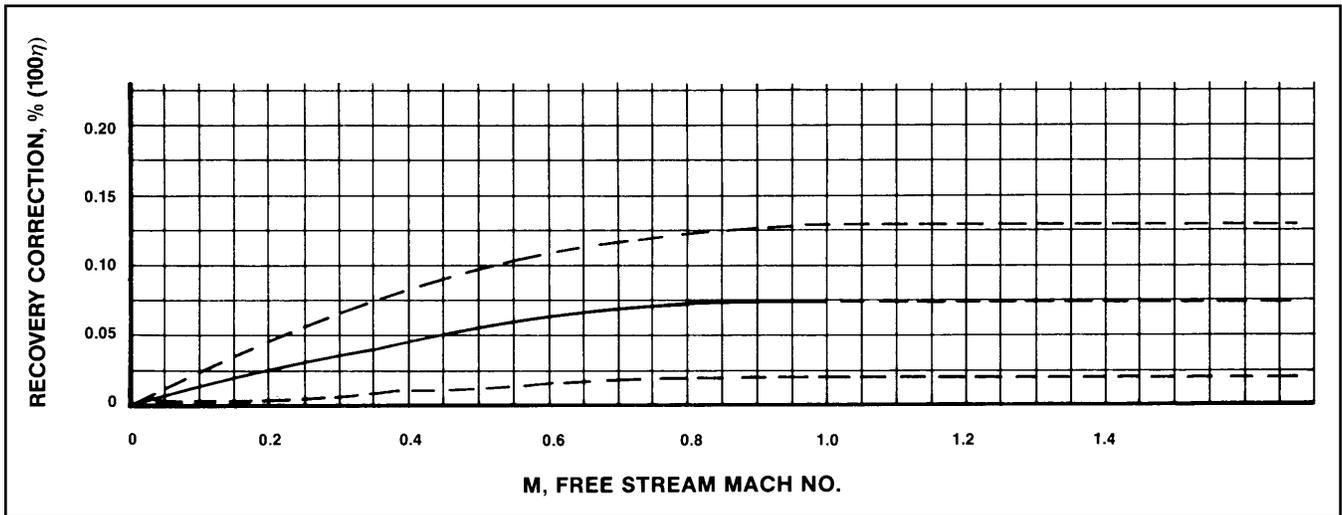
Figure 20: Wind Tunnel Data; Non-deiced Model 102 Recovery Corrections
