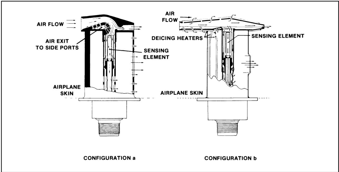
Figures 10-A, -B: Internal Configurations of the Model 102 Deiced Sensors Showing Boundary Layer Control, Particle Separation Path, and the Hermetically Sealed Sensing Element
