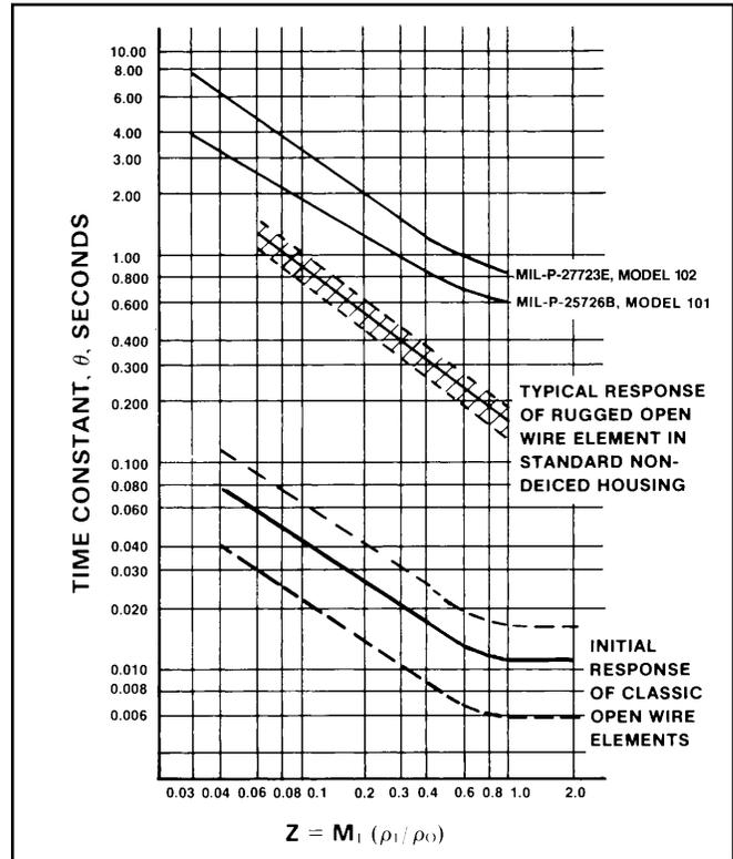
Figure 23: Wind Tunnel Data; Time Constant of Open Wire Elements and MIL-SPEC Elements
