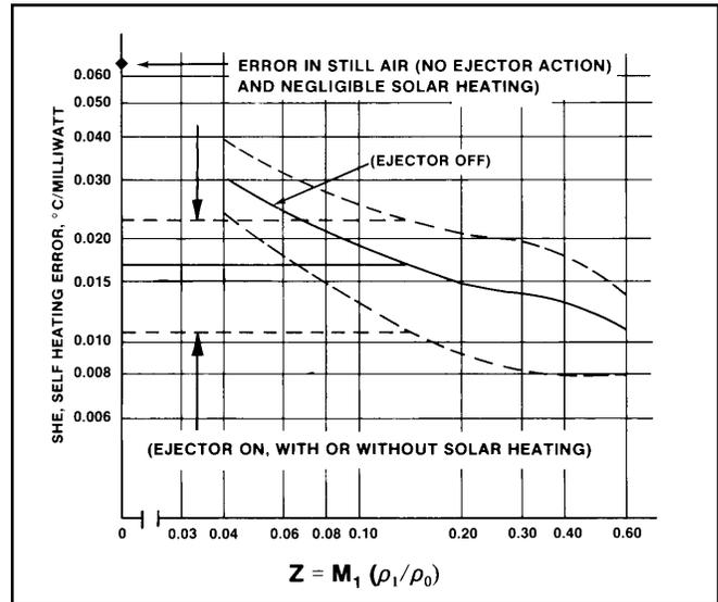
Figure 17: Wind Tunnel Data; Ejector Model Self-heating Errors
