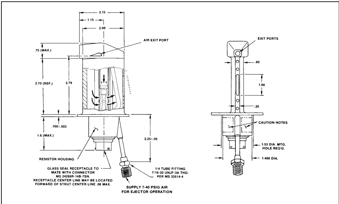
Figure 16: Ejector Model 102 Configuration
