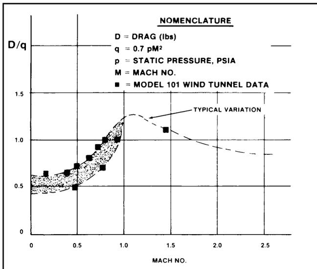
Figure 9: Wind Tunnel Data; Aerodynamic Drag of Model 101 Sensors
